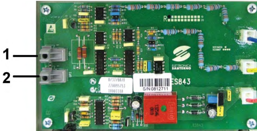
Figure 37: ES843 Bus-bar Voltage Acquisition Board
